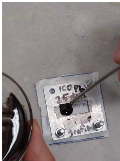
Figure 4.19: Graphite and coal powders are prepared until maximum value 3 % inside the mixture of epoxy.
