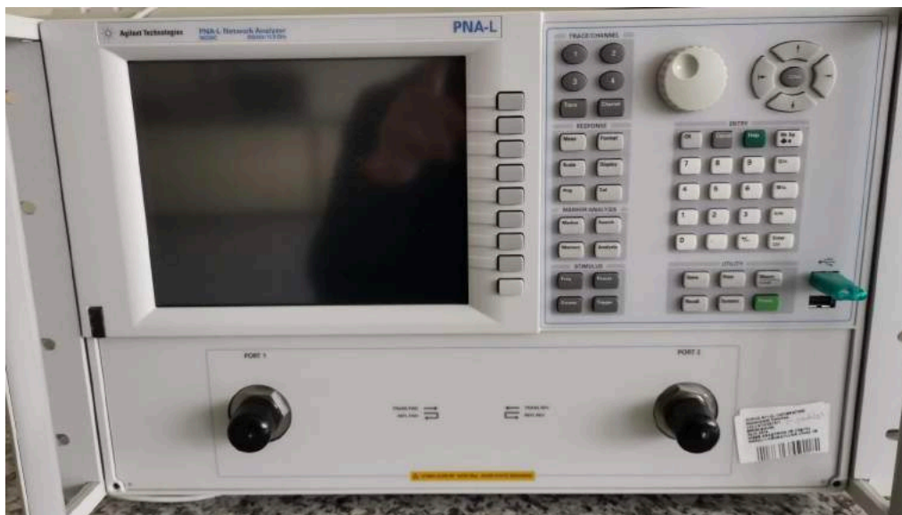
Figure 3.3: Vector Network Analyzer N5230C 300 kHz - 13.5 GHz by Agilent Technologies was used in between 8 and 12 GHz.
