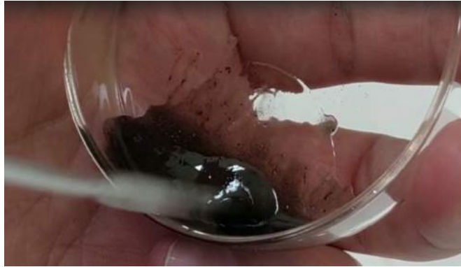
Figure 4.19: Graphite and coal powders are prepared until maximum value 3 % inside the mixture of epoxy.
