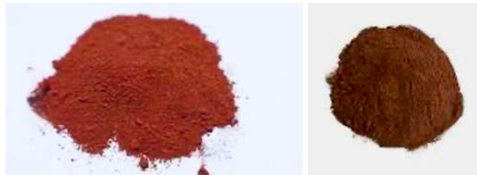
Figure 4.13: Comparison of lead oxide powder. The smaller particle size (below 25 micron) looks much more reddish (left) and the greater particle size (above 135 micron) looks completely brown.
